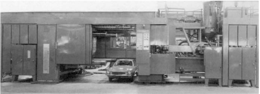
Figure 2.20 This 2500 ton hydraulic machine has a special retractable tie-rod system; the car is included for scale.
