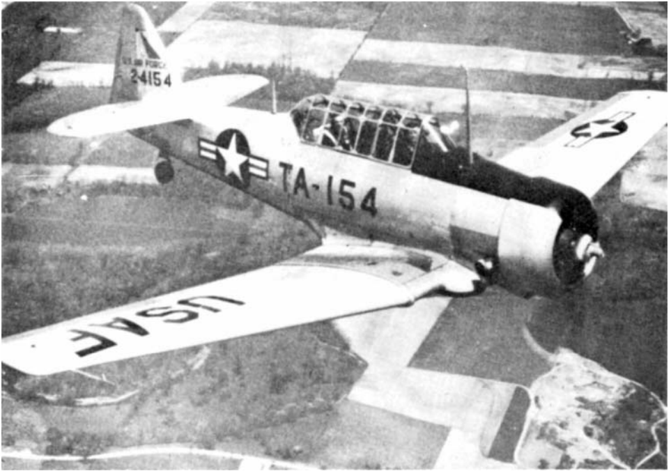
Figure 12.3 Final flight tests of the Air Force AT-6 (all RP, hand layup); later, during 1953, BT-15 airplanes were fabricated in Long Island.
