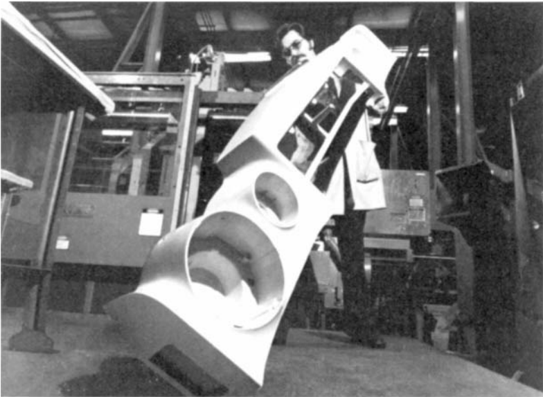
Figure 12.25 Automobile front panel injection-molded from short glass fiber-TS polyester resin compound.
