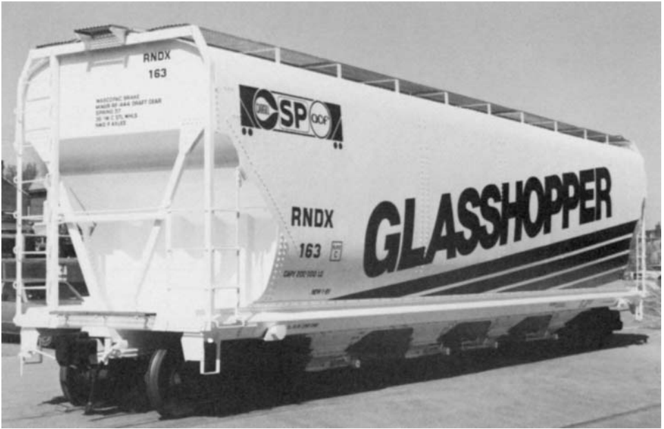
Figure 12.23 Glasshopper: the first railcar using RP by Cargill Inc./Southern Pacific and ACF Industries. It had two major advantages: a lower tare weight (8000lb (3632kg) lighter than steel cars) and corrosion resistance (principally against the contents to be carried, such as fertilizers) [3].
