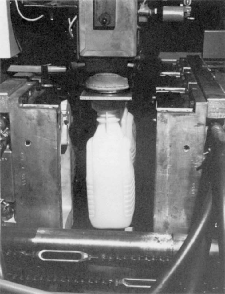
Figure 4.10 A multiple continuous extrusion head (three parisons) blow molding three containers simultaneously in a shuttle clamping system.
