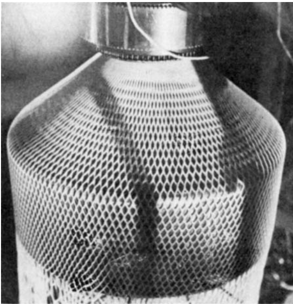
Figure 3.43 Netting exits the die and undergoes postextrusion stretching.
