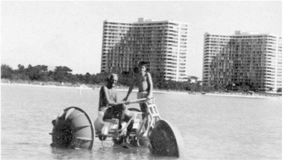
Figure 4.2 Aquacycle: its blow-molded PP wheels incorporate paddles and fins on their sides; they operate most efficiently.
