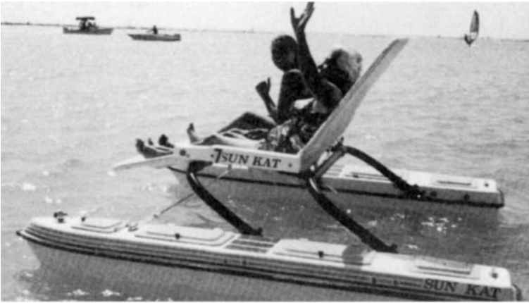
Figure 1.43 Injection-molded plastic and RP open layup produces the leisure boat.
