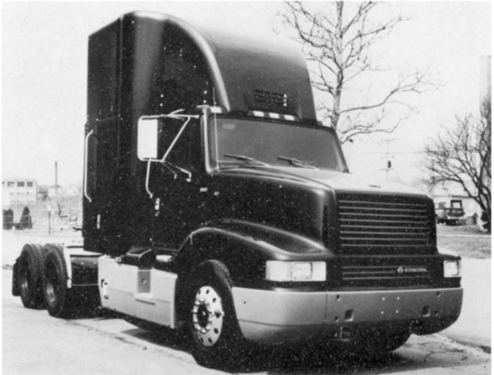
Figure 4.3 Truck fascia: multiple-extrusion blow-molded PP.
