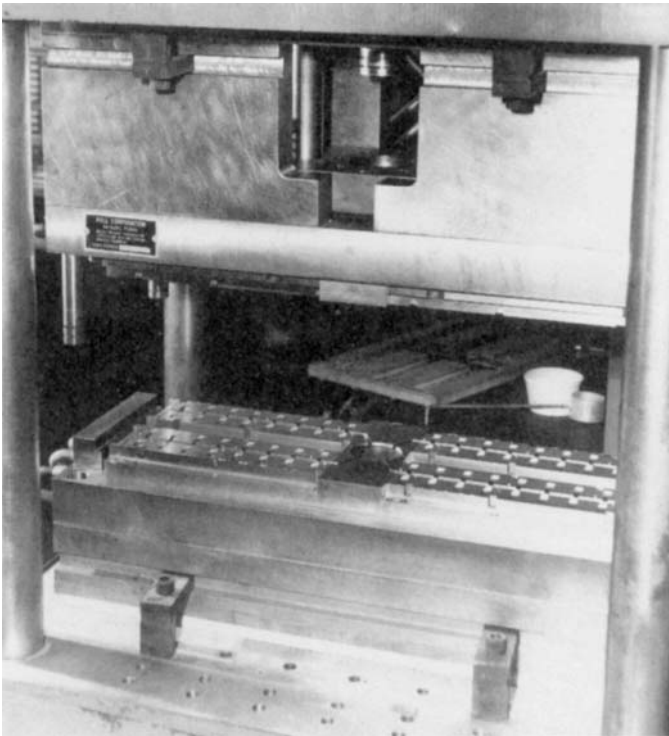
Figure 8.3 Front view of a 64-cavity mold (with integrated circuits) showing layout, top-transfer pot, and plunger used in a transfer molding system. (Courtesy Hull Corp.)
