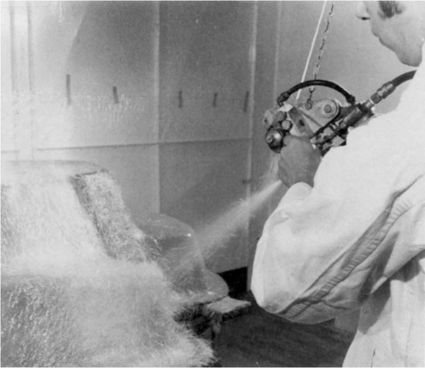
Figure 12.14 Sprayup process for composites.
