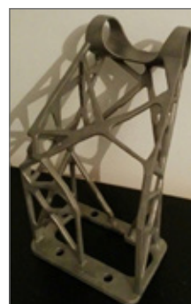
Satellite bracket redesigned for additive manufacturing with topology optimisation: left after topology optimisation, middle after smoothing and right after manufacturing (Courtesy of Poly-Shape)
