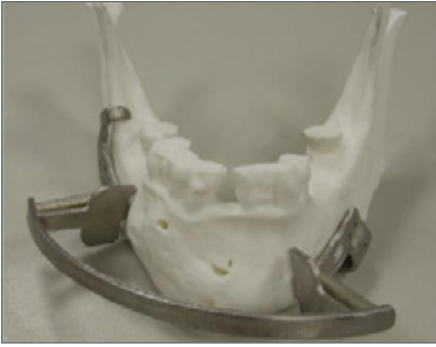
316L Surgical guide made by Laser Beam Melting (Courtesy of IK4-Lortek)
