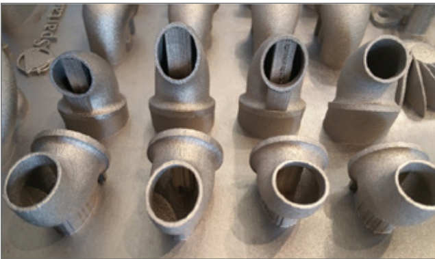
Different part positions and orientations and their influence on the location and importance of support structures (Courtesy of Spartacus 3D)
