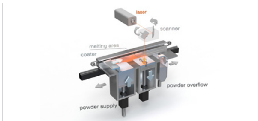
Inside a Laser Beam Melting Machine (Courtesy of Concept Laser GmbH)
