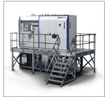
SLM800 by SLM Solutions GmbH Platform size: 500mm x 280mm x 850mm
