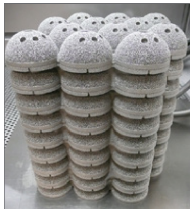
Ti6Al4V implant (acetabular cup) with high specific surface design for improved osseointegration. (Courtesy of ARCAM)
