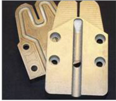
Tooling insert by Laser Beam Melting (Courtesy of BMW)
