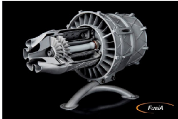
Gas turbine demonstrator (diameter 250 mm and length 600 mm), by assembling parts made by Selective Laser Melting with Al-, Ti- and Ni-base powders for integration of functions, reduced number of parts, weight saving and increase of performance (Courtesy of FusiA)
