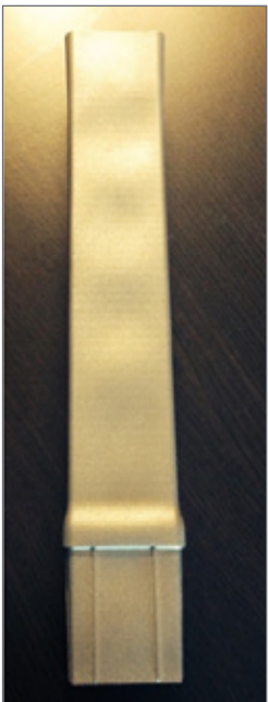
Bike frame component showing buckling effect due to too high length to height ratio. (Courtesy of Renishaw)
